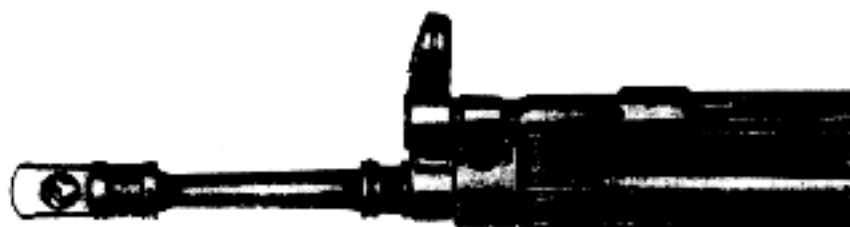
Fig. 58: Blank attachment mounted
